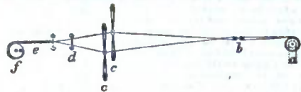
FIG. 26.—Section of Plain Web in Process of Weaving on the Loom.
